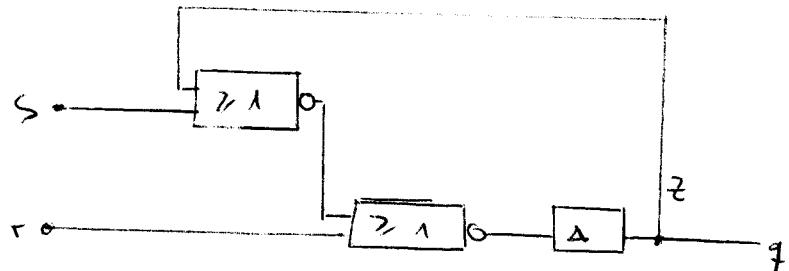
$$\begin{cases} s(t) = 1 \\ z(t + \Delta) = 1 \end{cases} \left. \begin{array}{l} \text{bleibt stabil, bis} \\ r(t') = 1 \end{array} \right.$$
