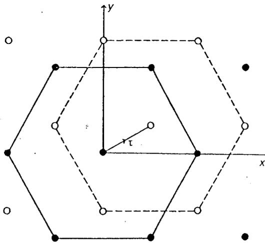
Fig. 1.9. The hexagonal closed-packed structure  $D_{6h}^4$ . The full and empty circles represent nuclei lying in the planes  $z=0$  and  $z=\frac{1}{2}c$  respectively.
