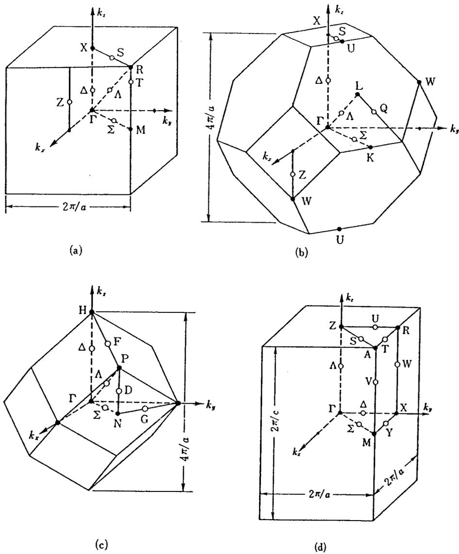
**Fig. 11.7.** Brillouin zones for (a) simple cubic, (b) face-centered cubic, (c) body-centered cubic, and (d) simple tetragonal lattices
