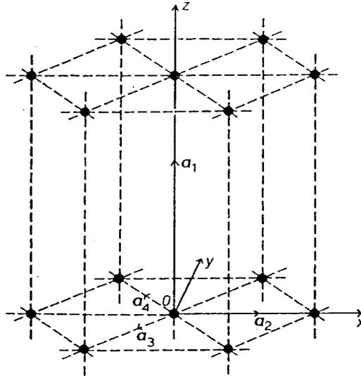
Fig. 1.8. The simple hexagonal lattice  $\Gamma_h$ . (Symmorphic)
