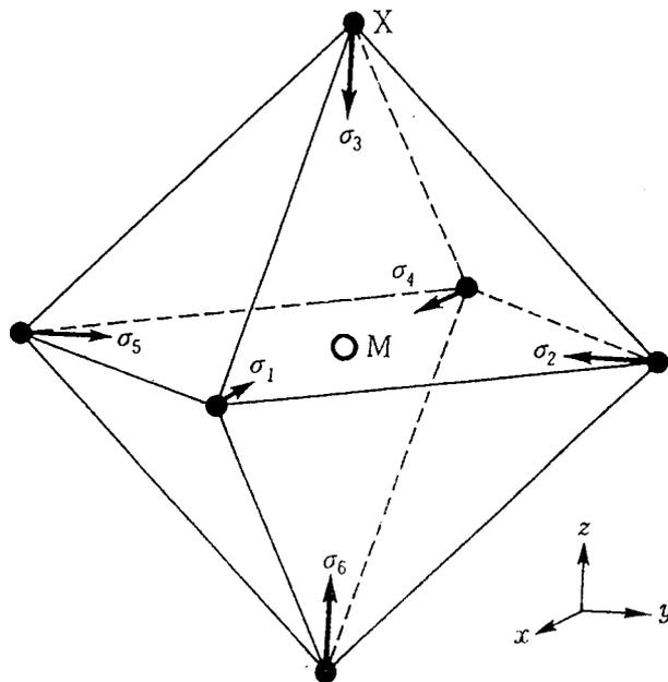
Fig. 9.6.  $\sigma$  orbitals of the six ligands in an  $MX_6$  complex ion
