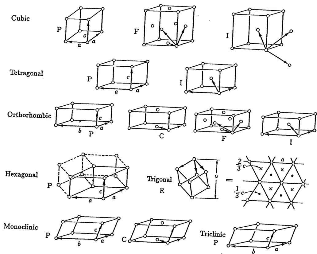
**Fig. 11.6.** The fourteen Bravais lattices. The arrows show the fundamental period vectors commonly used
